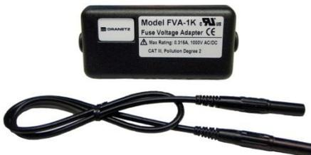
Inline fuse adapter for one voltage channel, 4mm connector, 1000V MAX.
