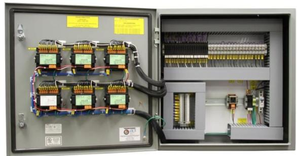
BCEM is an enclosure that holds up to 6, 12 or 24 ES210, ES230s, ES220 and ES230 meters (sold separately). Includes 120V power outlet, fused voltage connections, CT shorting blocks and internal wiring.
