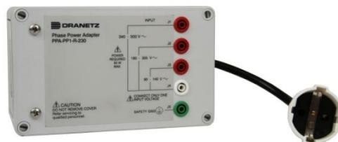
Power the instrument from the phase being measured. For circuits from 90V to 500Vrms.
